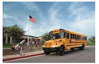
The new 35' 08" bus body option provides customers flexibility by allowing expanded capacity up to 83 passengers, or additional seat spacing configurations for more passenger room.
