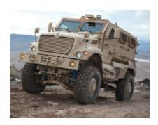
The enhanced MaxxPro Dash with DXM independent suspension offers added mobility for off-road travel while still providing warfighters with Category I MRAP survivability protection. A number of other added features that are included on the enhanced Dash include insulation and door upgrades, as well as an inclinometer, which acts as a level and measures side slope during vehicle operation.
